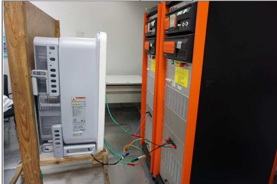
SURGE TEST (AC Power Port)
