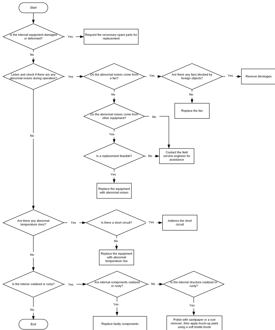
Figure 7-8 Workflow for System Status and Cleanliness Inspection (Every Two Years)
