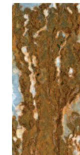
Hot dip galvanized 20µm after 6 weeks
