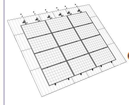
1 MOUNT THE TOP SOLAR PANEL ONTO THE RAILS
